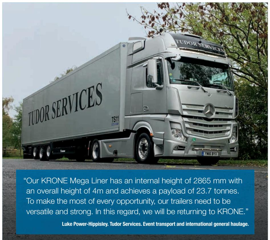
“Our KRONE Mega Liner has an internal height of 2865 mm with an overall height of 4m and achieves a payload of 23.7 tonnes. To make the most of every opportunity, our trailers need to be versatile and strong. In this regard, we will be returning to KRONE.”
